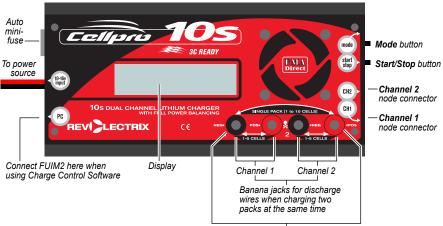
Banana jacks for discharge wires when charging one pack, or insert Plug Blocker when not charging through discharge wires
