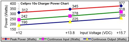
Peak Power = Maximum input power charger draws for first 3-5 minutes of charge.
